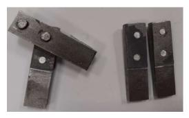
Fig. 9. Two methods of destroying hybrid lap joints of bended samples
