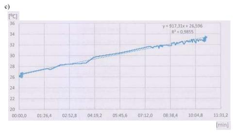
Fig. 9. Results of the measurements of the temperature of the actuating system during lapping of steel elements: a) in the initial moment, b) after  $10 \text{ min (n_t = 80 min^{-1}), c)}$  graph showing the increase of the temperature in time (on average by  $0.67^{\circ}\text{C/min}$ )
