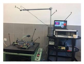
Fig. 1. General view of the test stand: 1 - single-disc lapping machine, 2 - thermal vision camera, 3 - camera stand, 4 - guiding ring rotational speed sensor, 5, 6 - device recording the rotational speed of the lapping disc and guiding rings, 7 - laptop computer
