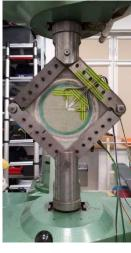
Fig. 10. Fixing the sample in the testing machine
