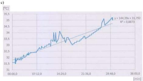
Fig. 12. Results of the measurements of the temperature of the actuating system during lapping of steel elements: a) in the initial moment, b) after 30 minutes ( $n_t = 80 \text{ min}^{-1}$ ), c) graph showing the increase of temperature in time
