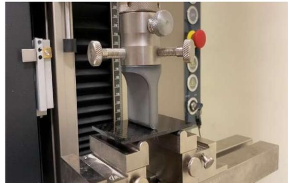
Fig. 10. Bending flexural strength test
