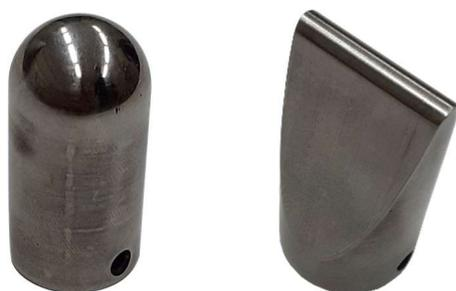
Fig. 1. Shapes of 'impactors' used in the tests
